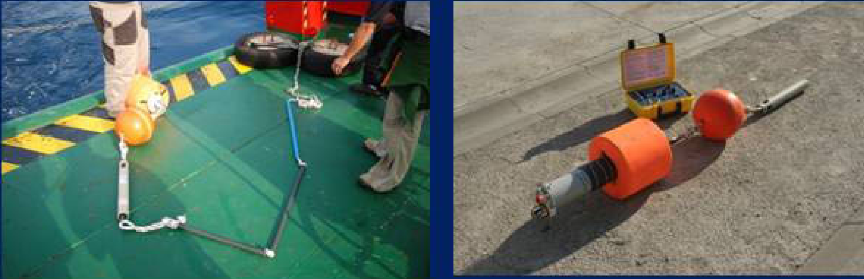
Figure 3: Mooring System: EAR attached to the acoustic release device (7986 LRT, Sonardyne Ltd, Hampshire, UK). The system was moored on the seafloor with a sinker weight of 200kg and a floating line of 2 buoys (12kg).
