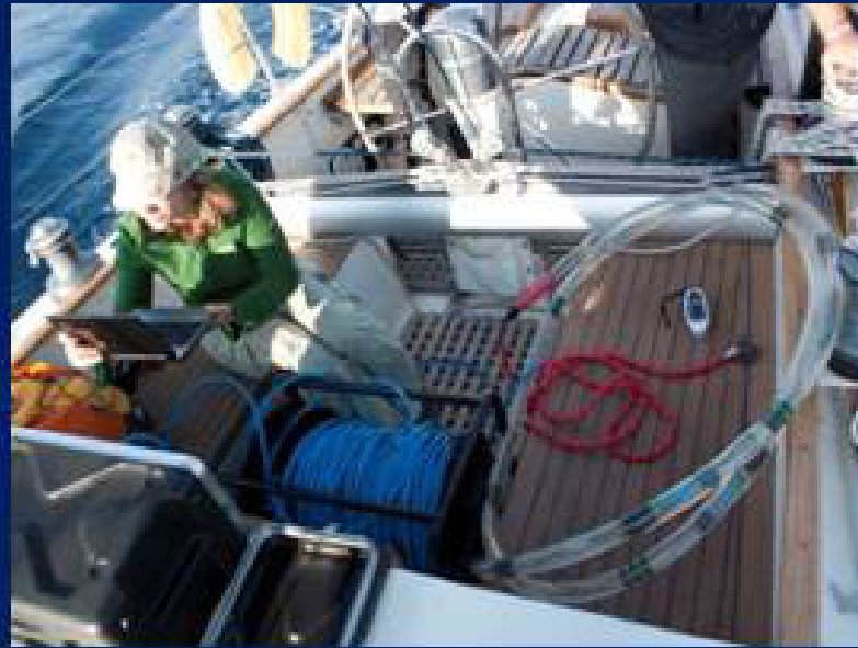
Figure 5: The registration chain: Towed array hydrophone, an amplifier ROLLS MX54s ProMix Plus, a converter from analog to digital signal E-MU USB 2.0, a low frequency filter and a computer with specialized software (Ishmael 2.0 (NOAA), whistles (IFAW), Rainbowclick (IFAW)) that allows the visualization of the sound and its interpretation by the observer.
