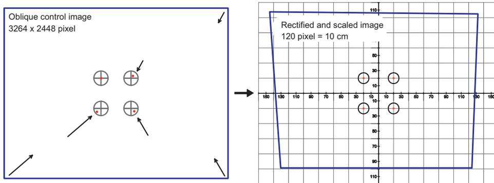
Fig. 3. Simplified scheme of image rectification and scaling processes. The coordinates estimated were used for resampling, surface calculations and for sizing species.
