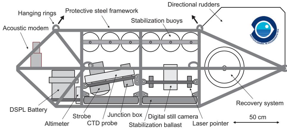
Fig. 2. Diagrammatic side-view of the TFS-2 photogrammetric sled showing the location of its main technical components.
